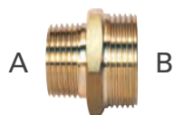
Nipplo ridotti M/M in ottone con filettatura maschio ISO 228 G a battuta piana (B) e filettatura maschio conica EN 10226 R (A) Brass M/M reduced nipples with ISO 228 G male thread with plane end (B) and EN 10226 R male taper thread (A)
